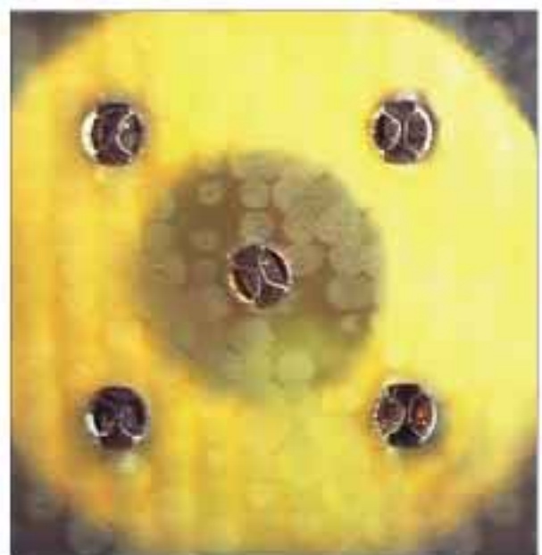
Cross section of press fit pins pressed into the PCB
