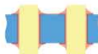
Excess solder causes "bridging" between pads or leads
