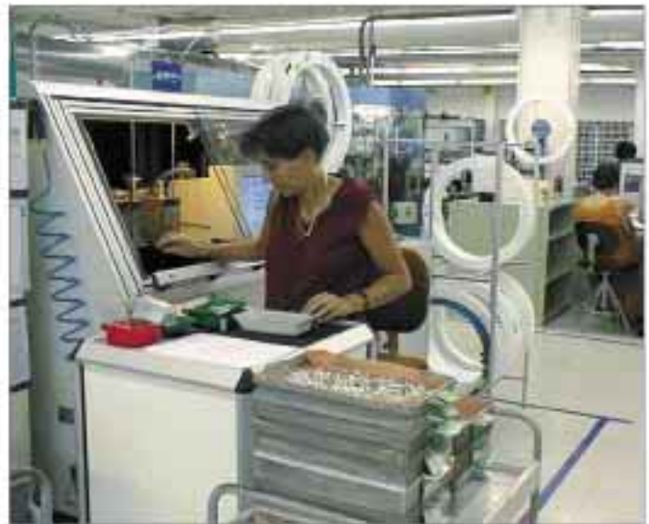
Connector manufacturing : press fit pins assembly line
