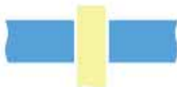
Dewetting case (wave soldering)
