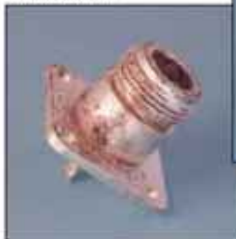
Silver plated receptacle after salt mist exposure ▼
